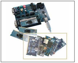
including the REva evaluation board, microcontrollers, embedded RLink JTAG in-circuit debugger/programmer and Raisonance Integrated Development Environment (RIDE).
